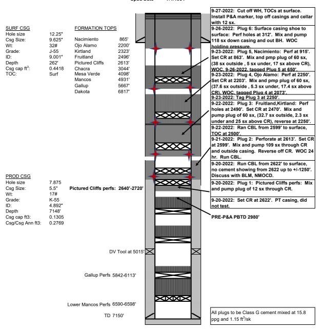
P&A NOTE: On 9-22-2022: CR at 2599' was not capped with cement. Plug 2 was pumped, and reverse circulated to run CBL from 2599'. After CBL, holes were perfed at 2490' and Plug 3 pumped before it was realized that no cement had been pumped above the 2599' CR. NMOCD and BLM approved leaving the plugs as pumped.
