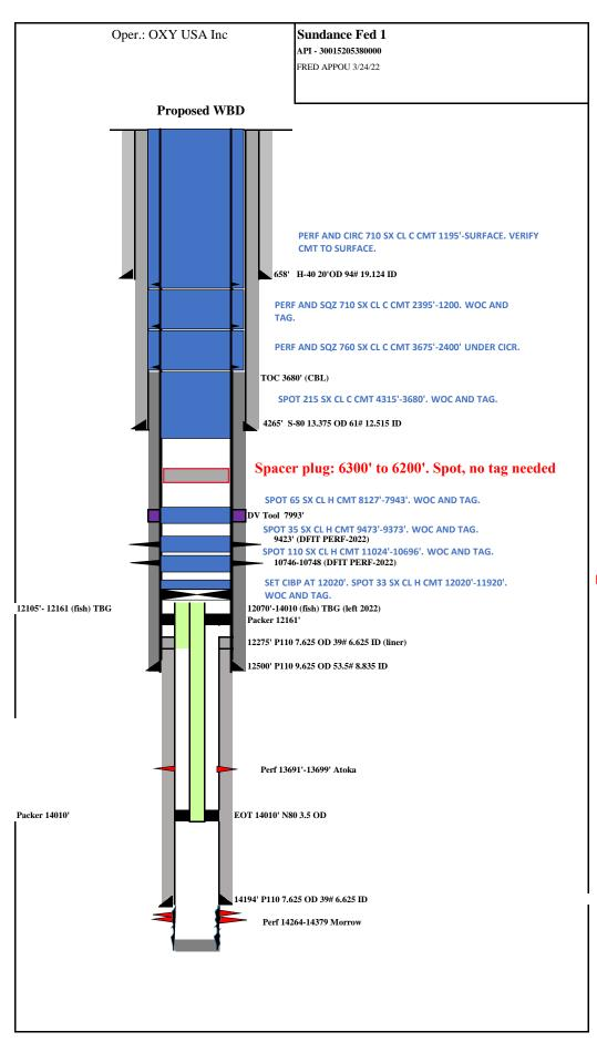
When staging plugs(from 4315' to surface) start the upcoming plug where the prior plug was tagged
