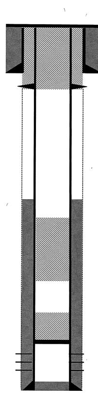
$8\mbox{-}5\mbox{/}8"$  28# casing @ 149'. Cemented with 150 sks Class B cement . Circulated cement to surface.
