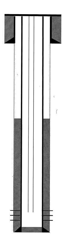
8-5/8" 28# casing @ 149'. Cemented with 150 sks Class B cement . Circulated cement to surface.
