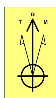
**Azimuths to Grid North** True North: -0.38° Magnetic North: 6.09°
