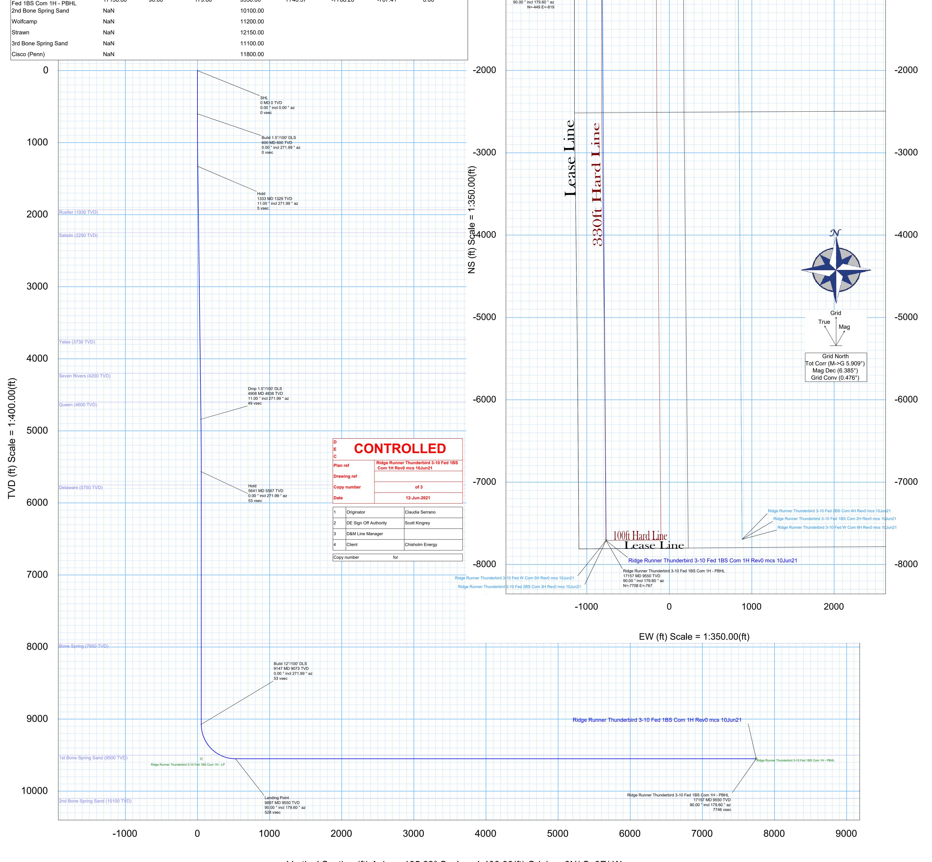
Vertical Section (ft) Azim = 185.69° Scale = 1:400.00(ft) Origin = 0N/-S, 0E/-W
