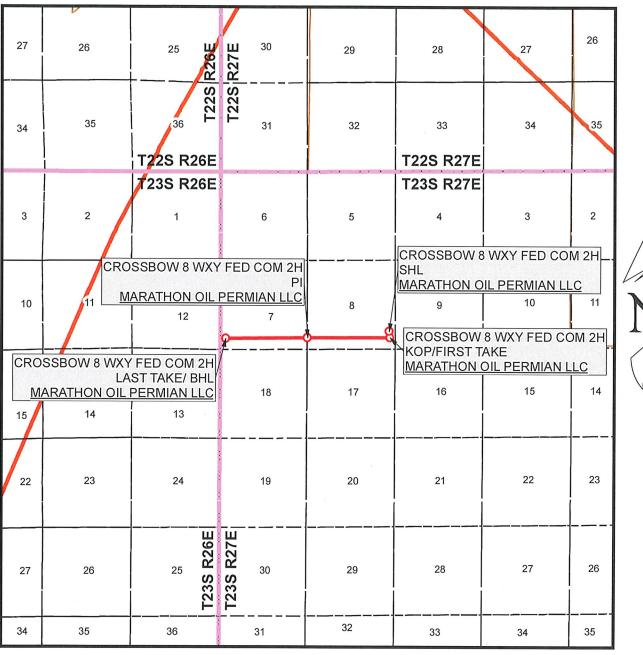
SEC. 8 TWP. 23-S RGE. 27-E SURVEY: N.M.P.M. COUNTY: EDDY OPERATOR: MARATHON OIL PERMIAN LLC DESCRIPTION: 1029' FSL & 378' FEL ELEVATION: 3158' LEASE: CROSSBOW 8 FED COM U.S.G.S. TOPOGRAPHIC MAP: OTIS, NM.
