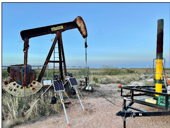
3) Foster #001 (30-025-07968) – Methane Flow Monitoring Rig Up
