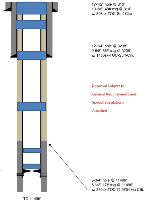
OXY USA Inc. – Proposed Plugging Procedure Roadside Federal #1 API No. 30-015-31277
