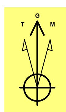
Azimuths to Grid North True North: -0.36° Magnetic North: 6.20°
