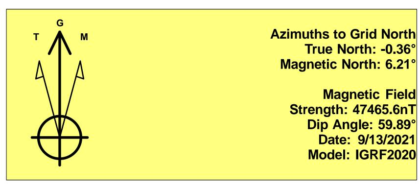
To convert a Magnetic Direction to a Grid Direction, Add 6.21° To convert a Magnetic Direction to a True Direction, Add 6.56° East To convert a True Direction to a Grid Direction, Subtract 0.36°
