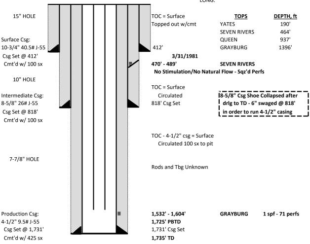
After well was drilled to 818' & 8-5/8" csg set - Seven Rivers compl'n attempted Perfed 470-489' - No Natural Flow - No Stimulation. Perfs Squeezed. Well was drilled to TD @ 1735'. 8-5/8" casing shoe collapsed & 6" swedge was used at 818' in order to run 4-1/2" casing.
