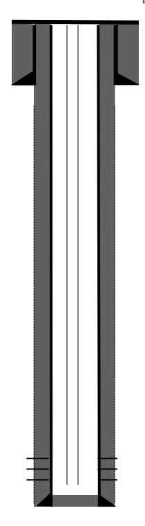
8-5/8" 24# casing @ 135'. Cemented with 100 sks Class B cement w/2% CaCl2 . Circulated cement. Hole size: 12  $^{1}\!4"$
