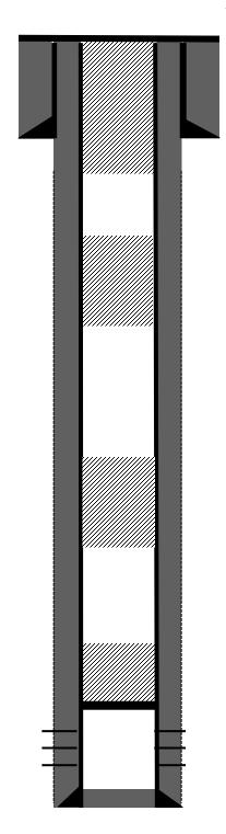
8-5/8" 24# casing @ 135'. Cemented with 100 sks Class B cement w/2% CaCl2 . Circulated cement. Hole size: 12  $\frac{1}{4}$ "
