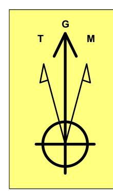
**Azimuths to Grid North** True North: -0.40° Magnetic North: 6.01°
