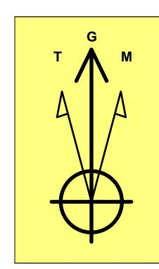
**Azimuths to Grid North** True North: -0.40° Magnetic North: 6.01°
