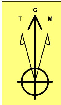
**Azimuths to Grid North** True North: -0.28° Magnetic North: 6.49°
