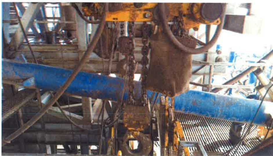
Figure 2: BOP Winch System
