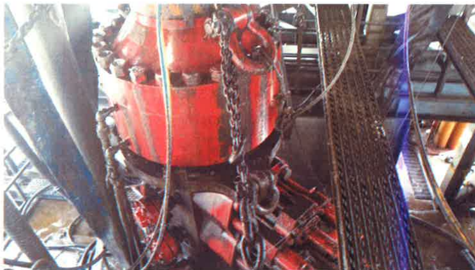
Figure 1: Winch System attached to BOP Stack
