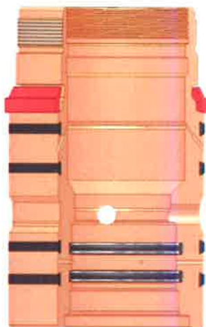
Annular packoff with both external and internal seals
