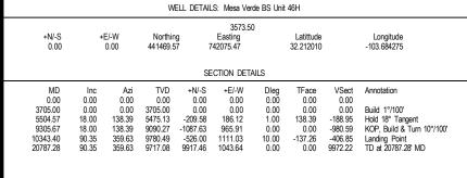
Azimuths to Grid North True North: -0.35° Magnetic North: 6.25°
