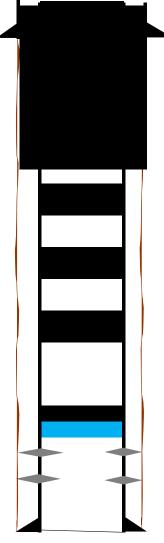
TD- 3848' PBTD- 3825' <u>Plug 6</u> 212 feet - Surface 212 foot plug 65 Sacks of Type I/II Cement
