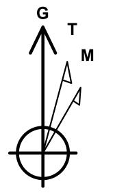
Azimuths to Grid North True North: 0.04° Magnetic North: 6.82°
