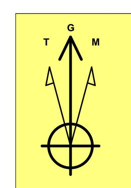
**Azimuths to Grid North** True North: -0.37° Magnetic North: 6.12°
