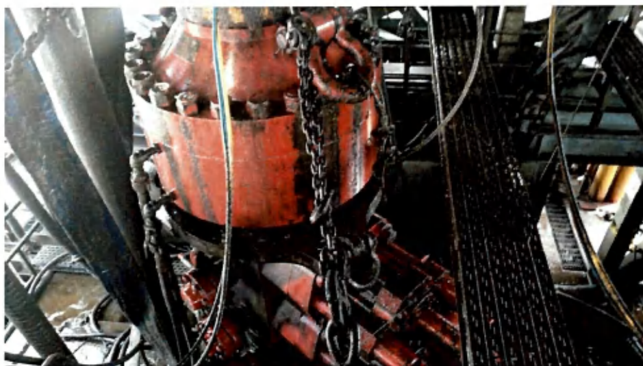
Figure 1: Winch System attached to BOP Stack
