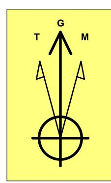
**Azimuths to Grid North** True North: -0.27° Magnetic North: 6.48°
