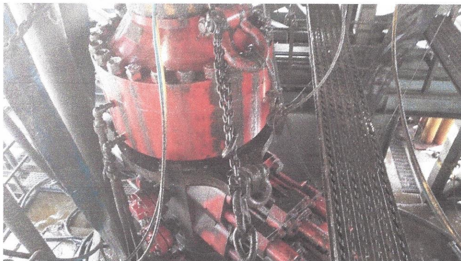
Figure 1: Winch System attached to BOP Stack
