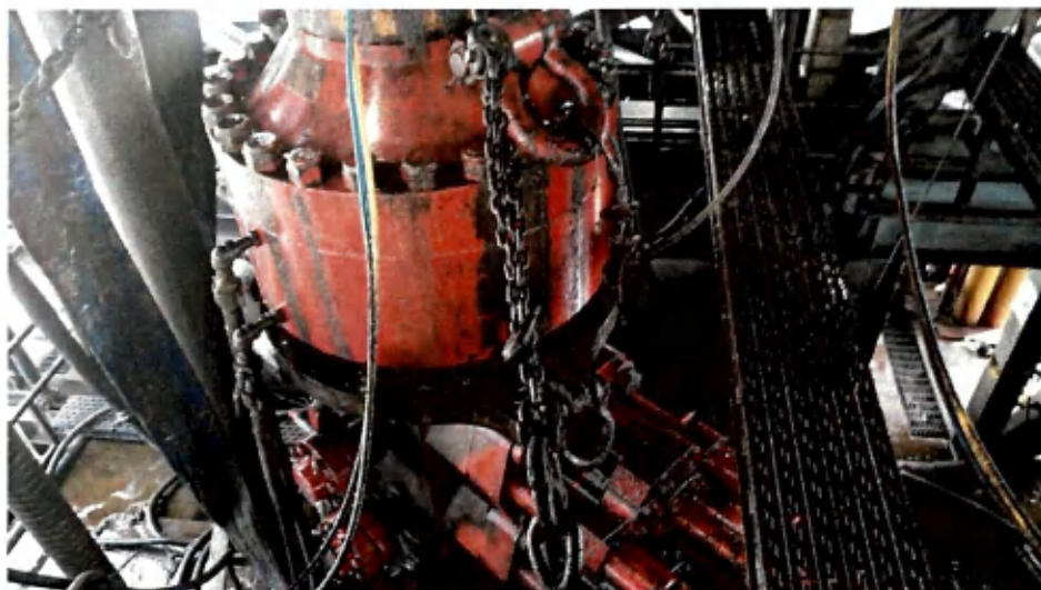
Figure 1: Winch System attached to BOP Stack
