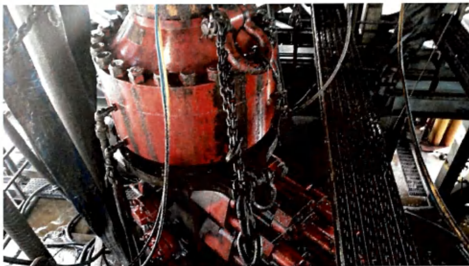
Figure 1: Winch System attached to BOP Stack
