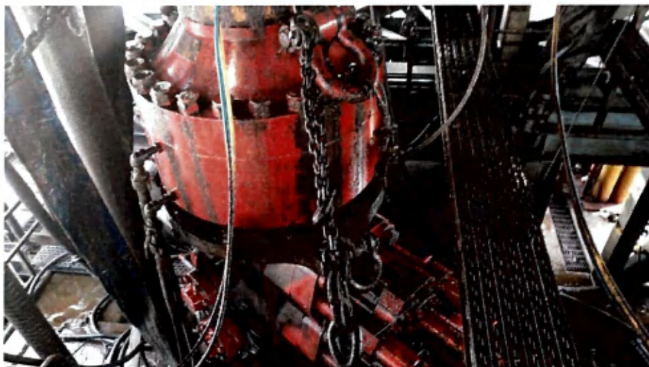
Figure 1: Winch System attached to BOP Stack
