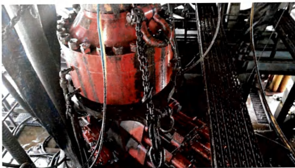
Figure 1: Winch System attached to BOP Stack
