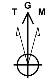
**Azimuths to Grid North** True North: -0.37° Magnetic North: 5.94°
