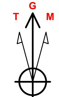
Azimuths to Grid North True North: -0.14° Magnetic North: 7.05°
