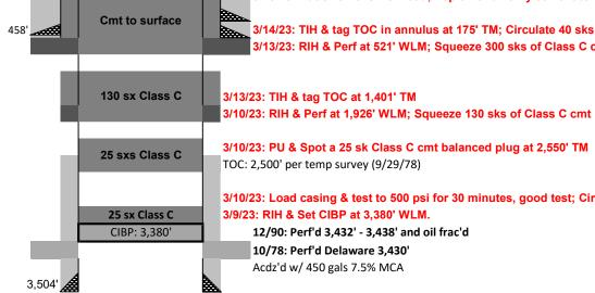
3/15/23: Cut & remove wellhead; Top off and verify cement to surface on all strings; Weld on dryhole marker; fill cellar and back drag location.
