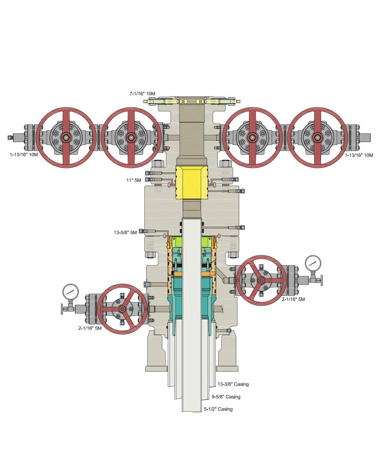
A multibowl wellhead may be used. The BOP will be tested per Onshore Order #2 after installation on the surface casing which will cover testing requirements for a maximum of 30 days. If any seal subject to test pressure is broken the system must be tested.
