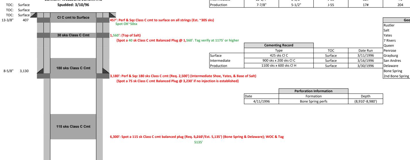
8,850': Set CIBP @ Spot 25 sks Class H cmt (Est. 8,647' / Req. 8,650') Leak test 500psi, 30mins
