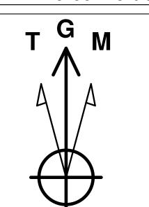
Azimuths to Grid North True North: -0.13° Magnetic North: 6.56°
