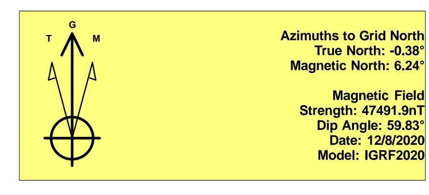
To convert a Magnetic Direction to a Grid Direction, Add 6.24° To convert a Magnetic Direction to a True Direction, Add 6.62° East To convert a True Direction to a Grid Direction, Subtract 0.38°
