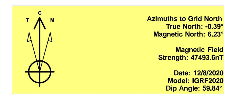
To convert a Magnetic Direction to a Grid Direction, Add 6.23° To convert a Magnetic Direction to a True Direction, Add 6.61° East To convert a True Direction to a Grid Direction, Subtract 0.39°
