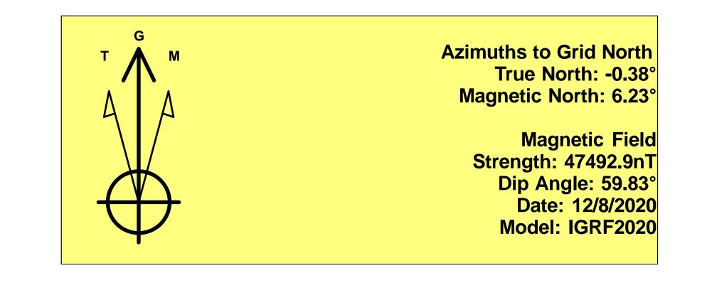
To convert a Magnetic Direction to a Grid Direction, Add 6.23° To convert a Magnetic Direction to a True Direction, Add 6.62° East To convert a True Direction to a Grid Direction, Subtract 0.38°
