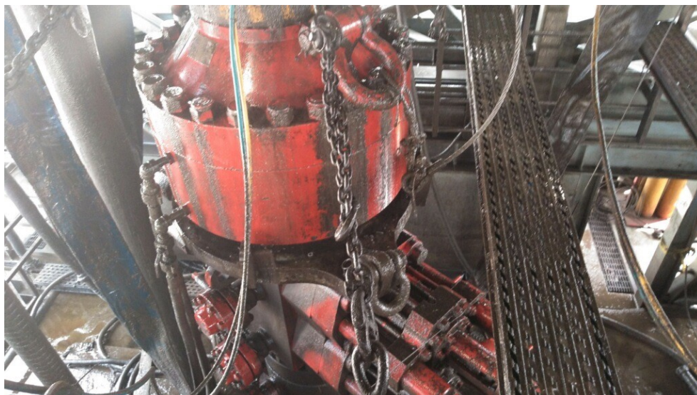
Figure 1: Winch System attached to BOP Stack
