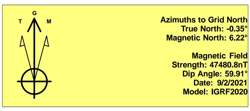
To convert a Magnetic Direction to a Grid Direction, Add 6.22° To convert a Magnetic Direction to a True Direction, Add 6.57° East To convert a True Direction to a Grid Direction, Subtract 0.35°
