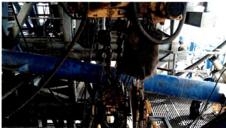
Figure 2: BOP Winch System
