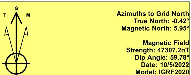
To convert a Magnetic Direction to a Grid Direction, Add 5.95° To convert a Magnetic Direction to a True Direction, Add 6.37° East To convert a True Direction to a Grid Direction, Subtract 0.42°
