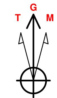
Azimuths to Grid North True North: -0.18° Magnetic North: 6.67°
