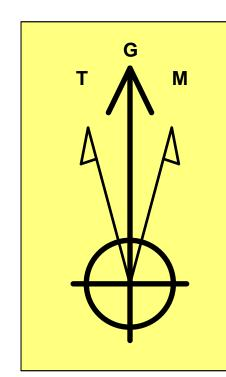
**Azimuths to Grid North** True North: -0.33° Magnetic North: 6.07°
