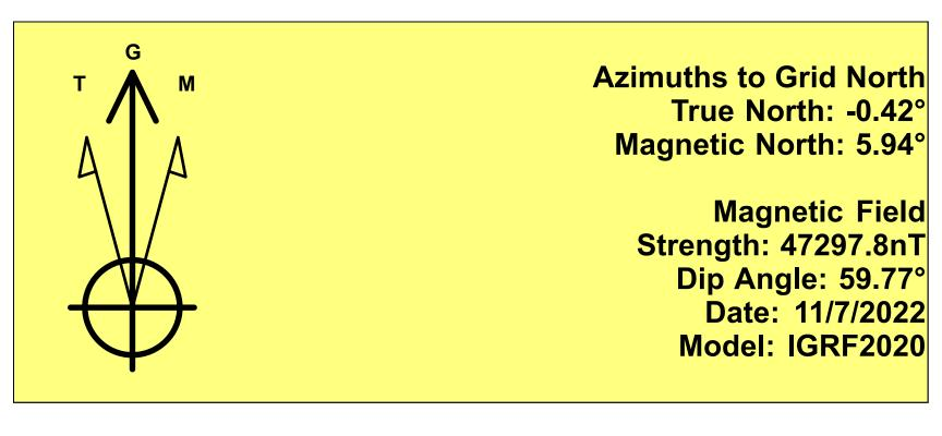
To convert a Magnetic Direction to a Grid Direction, Add 5.94° To convert a Magnetic Direction to a True Direction, Add 6.36° East To convert a True Direction to a Grid Direction, Subtract 0.42°
