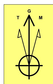
**Azimuths to Grid North** True North: -0.40° Magnetic North: 6.24°
