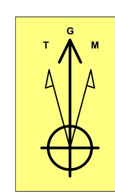
**Azimuths to Grid North** True North: -0.35° Magnetic North: 6.22°
