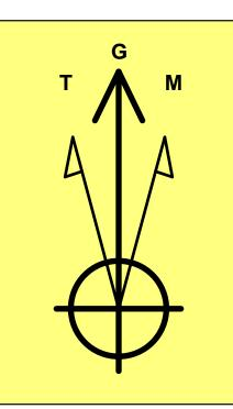
Azimuths to Grid North True North: -0.42° Magnetic North: 6.09°
