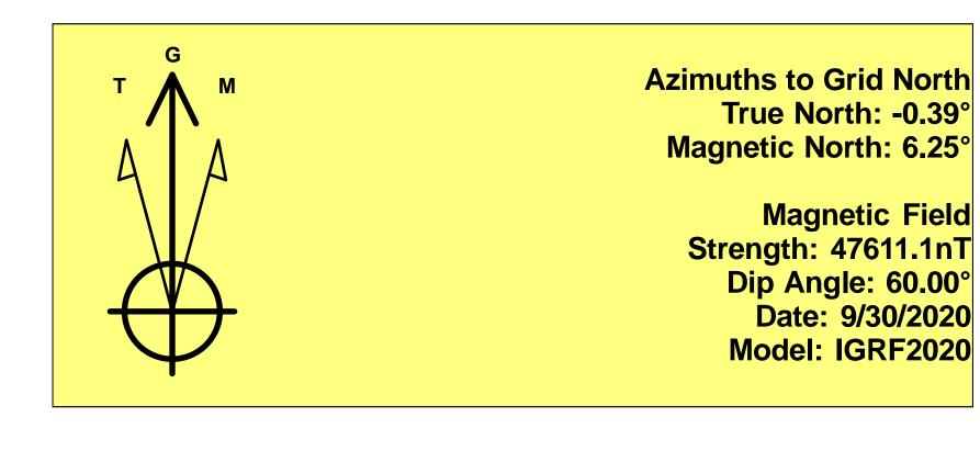
To convert a Magnetic Direction to a Grid Direction, Add 6.25° To convert a Magnetic Direction to a True Direction, Add 6.65° East To convert a True Direction to a Grid Direction, Subtract 0.39°
