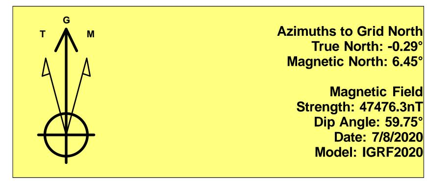
To convert a Magnetic Direction to a Grid Direction, Add 6.45° To convert a Magnetic Direction to a True Direction, Add 6.74° East To convert a True Direction to a Grid Direction, Subtract 0.29°
