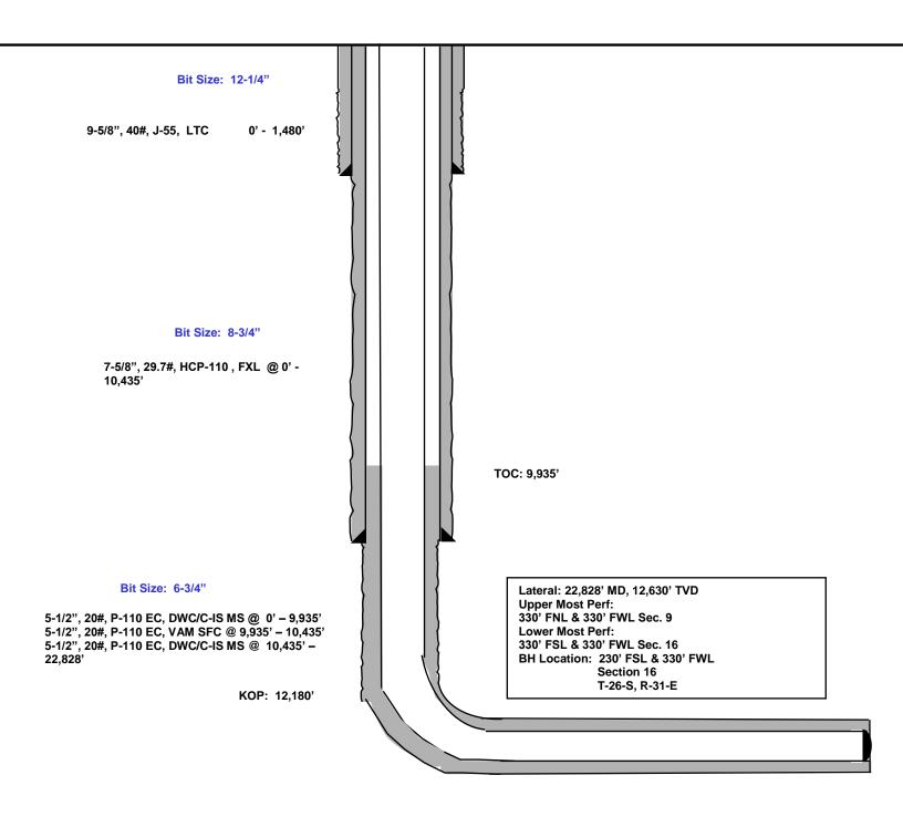
577' FSL 855' FWL Section 4 T-26-S, R-31-E Proposed Wellbore Design B KB: 3,315' GL: 3,290'
