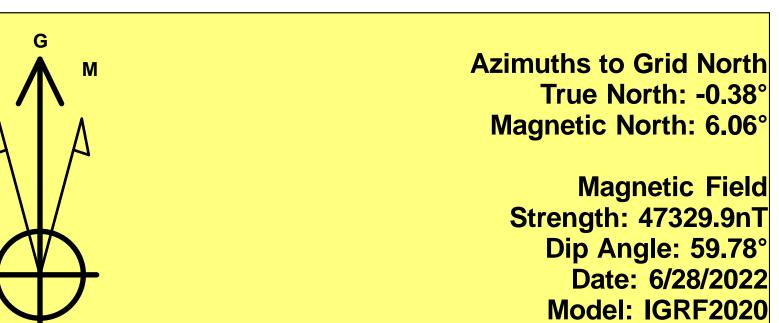
To convert a Magnetic Direction to a Grid Direction, Add 6.06° To convert a Magnetic Direction to a True Direction, Add 6.44° East To convert a True Direction to a Grid Direction, Subtract 0.38°
